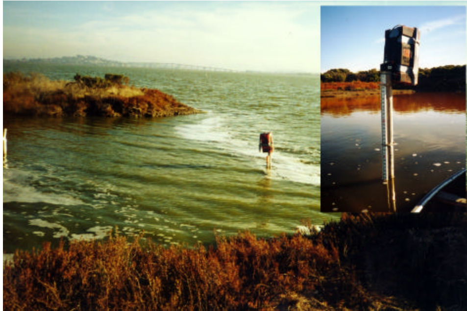
A conductivity probe to measure salinity and a pressure transducer to measure water surface elevation were attached to this staff gauge and connected to a data logger shown in the insert.
